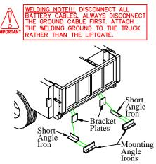
Figure 20: Lower bracket support.
