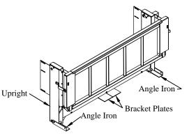
Figure 2: Complete liftgate.
