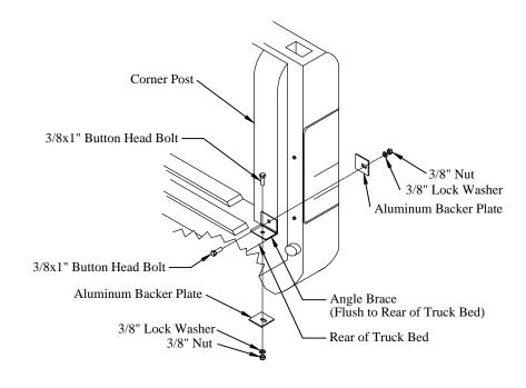
Figure 9: Angle brace location.
