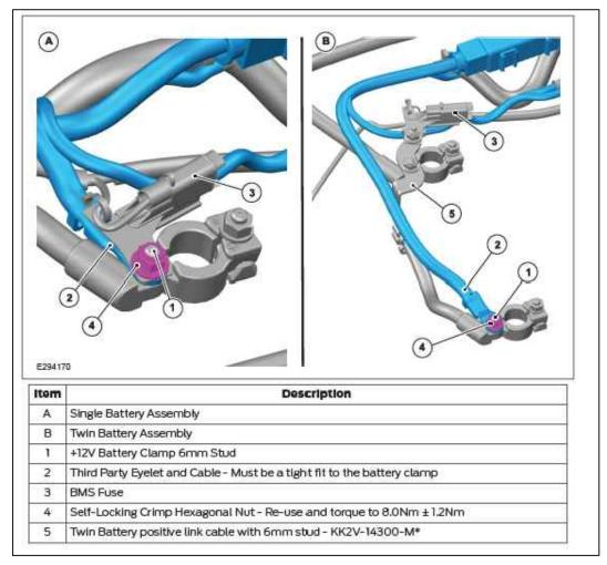
Figure 4: Battery diagram from 2020 Ford Transit Body and Equipment Mounting Manual (BEMM).
