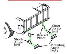
Figure 20: Lower bracket support.
