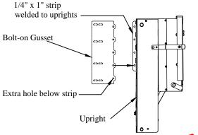
Figure 5: Liftgate requiring bolt-on gussets ( shown).
