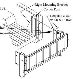
Figure 13: Mounting bracket and liftgate.
