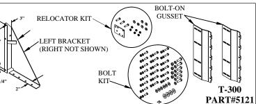
Table 1: T-300 Parts List. DESCRIPTION QTY. PART NO. Standard Pickup Bracket Bolt Bag Kit 9094 T-300 Left Corner Bracket 5184 T-300 Right Corner Bracket 5185 5160 Dodge Spare Tire Relocator Kit 6343 Standard Bolt-on Gusset
