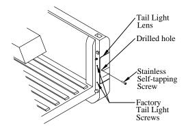
Figure 7: Tail light modification detail.
