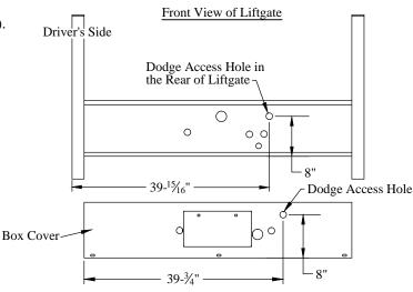
Figure 16: Spare tire access holes.
