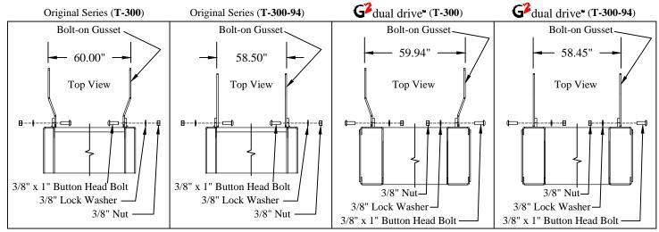
Figure 4: Top view of liftgate bolt-on gussets.
