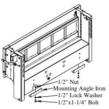
Figure 19: Mounting angle iron location.
