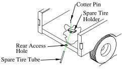
Figure 8: Spare tire tube detail.
