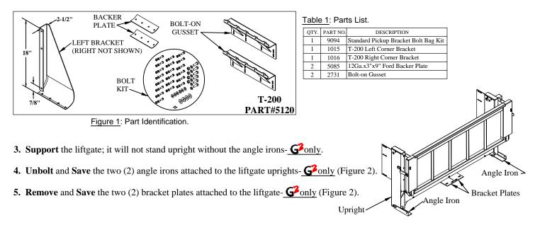
Figure 2: Complete liftgate (**G**<sup>2</sup> shown).
