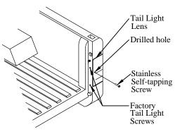
Figure 6: Tail light modification detail.
