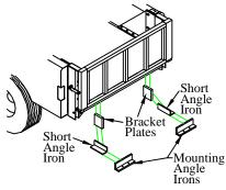
Figure 14: Lower bracket support.
