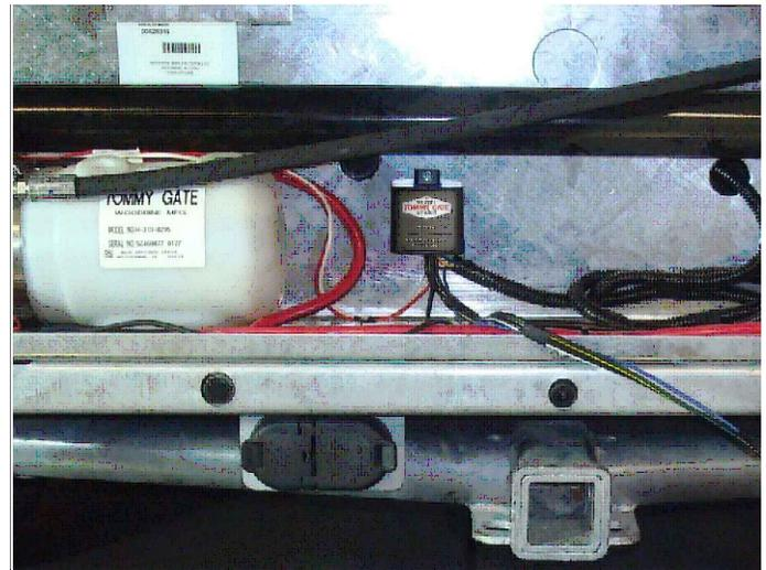
Figure 2: Relay location (G2 series shown).
